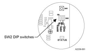
To configure the gas heating blower off delay settings, do the following:
