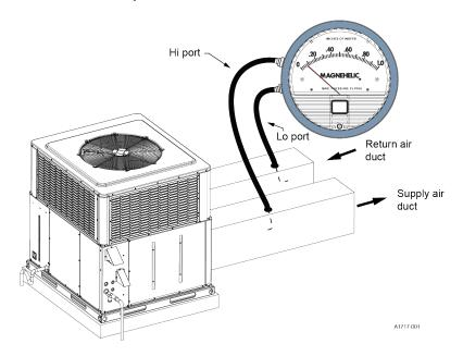
To measure the external static pressure, do the following:
