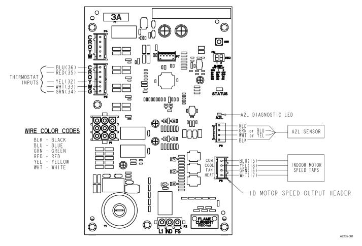
(i) Note: Figure 3 shows mitigation control wiring for PG3E48 and PG3E60 units. See Table 30 for an overview of the status LED and A2L diagnostic LED codes and troubleshooting guidance for A2L-related faults.
