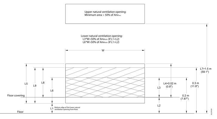
(i) **Note:** In Figure 2, only the shaded opening area below the 0.3 m point and above the floor covering (L2) counts as the effective natural ventilation area for the lower natural ventilation opening. To discern the effective natural ventilation area for the lower natural ventilation opening, you use the area between the 0.3 m point and whichever is higher of the floor covering height (L2) or the opening bottom edge height (L1).
