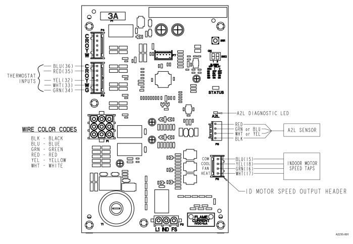
(i) Note: Figure 3 shows mitigation control wiring for PG3E48 and PG3E60 units. See Table 31 for an overview of the status LED and A2L diagnostic LED codes and troubleshooting guidance for A2L-related faults.
