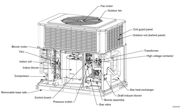
Figure 17: Unit components - PG3E42, PG3E48, and PG3E60 units with scroll compressor
