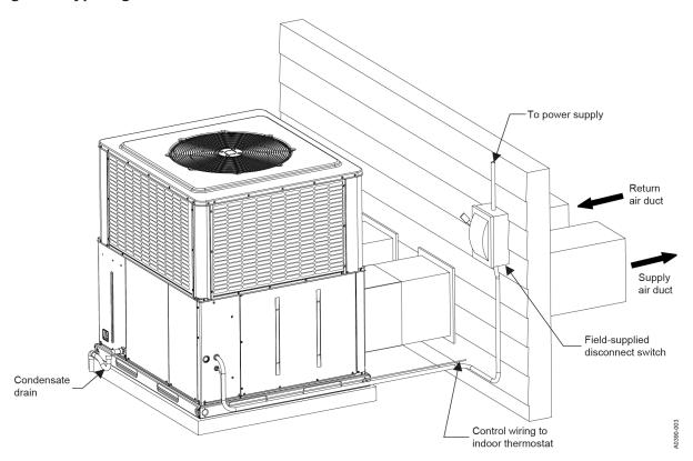
Figure 10: Typical installation on roof curb for unit
