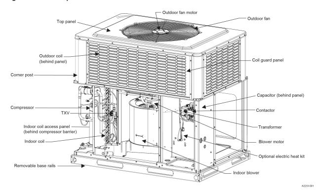
Figure 2: Unit components - PC3E48 and PC3E60 units
