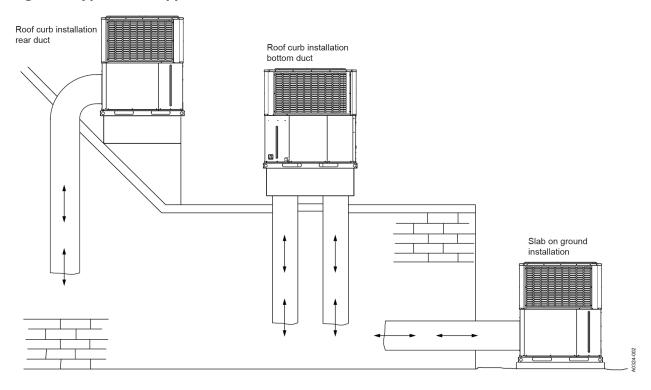
Figure 9: Typical ground installation on slab for unit
